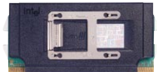
Example of an incorrectly installed retention clip
