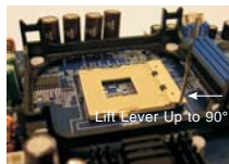
STEP 1: Lift The Socket Lever Up to 90°
