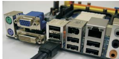
Connect the other end of the eSATAII device cable to eSATAII port of the I/O shield
