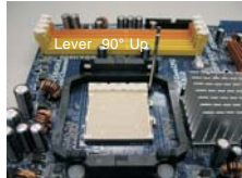
STEP 1: Lift Up The Socket Lever
