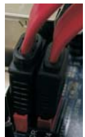
Connect the SATA data cables to both red eSATAII connector (eSATAII_BOTTOM) and orange eSATAII connector (eSATAII_TOP)
