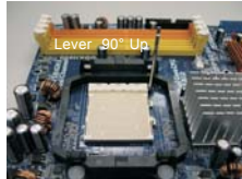
STEP 1: Lift Up The Socket Lever
