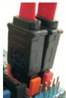
Connect the SATA data cables to both red SATAII connector (SATAII_RED (PORT 1)) and orange SATAII connector (SATAII_ORANGE (PORT 2))
