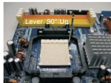
STEP 1: Lift Up The Socket Lever
