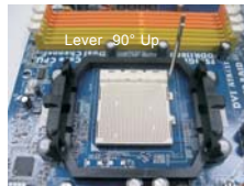
STEP 1: Lift Up The Socket Lever
