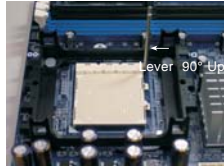
STEP 1: Lift Up The Socket Lever
