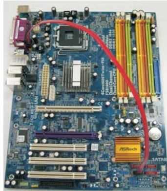
Connect the SATA data cable to the eSATAII connector (eSATAII)
