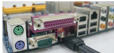
Connect the other end of the eSATAII device cable to eSATAII port of the I/O shield
