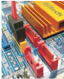
Connect the SATA data cable to the orange SATAII connector (SATAII_6 (Port5))
