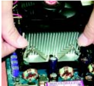
1. Hook one end of the cooler bracket to the CPU socket first.
