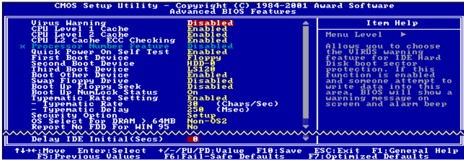
Figure 3-5. Advanced BIOS Features Setup Screen
