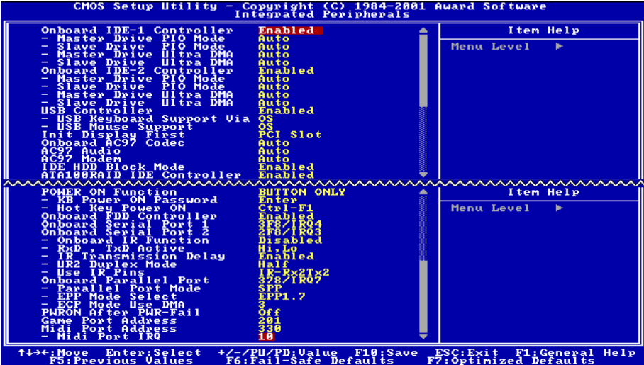
Figure 3-7. Integrated Peripherals Menu Screen
