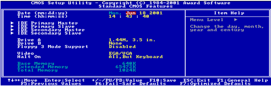
Figure 3-3. Standard CMOS Setup Screen Shot
