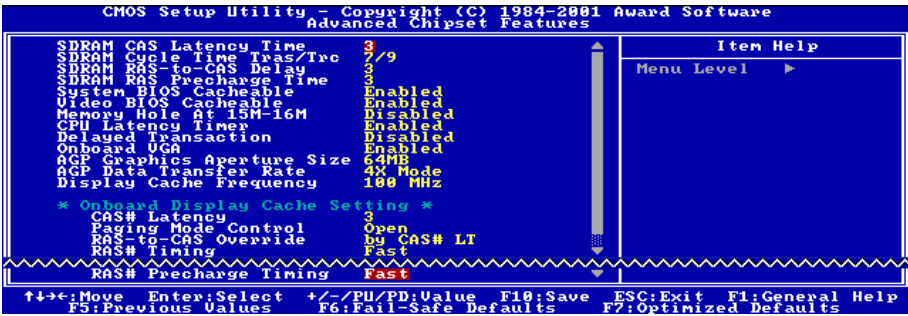
Figure 3-6. Chipset Features Setup Screen
