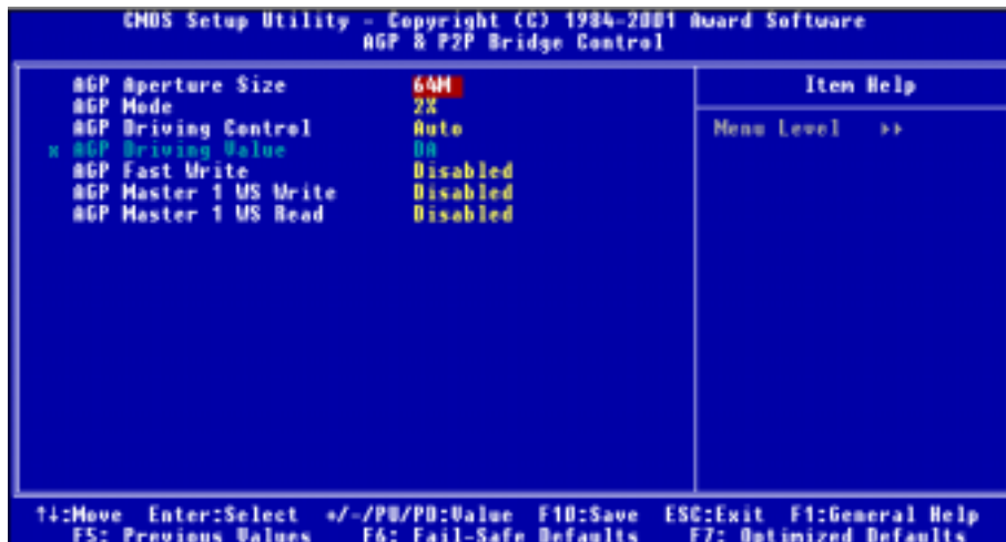
Figure 3-5C. AGP & P2P Bridge Control Screen
