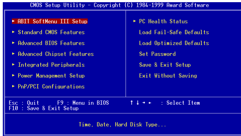
Figure 3-1. CMOS Setup Utility Main Screen Shot
