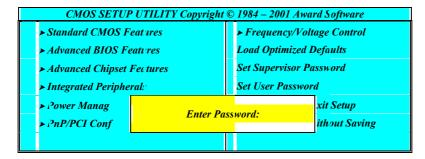
Now you can enter your password, after entering the password the menu will pop up again and will ask you to reconfirm the password. After entering and pressing [enter] the password will be stored to CMOS RAM and the password will be enabled.
