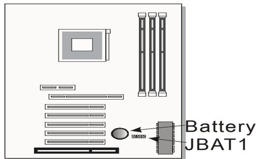
Normally JBAT1 will be in the 1-2 position, this will connect the battery to the southbridge of the chipset which contains the CMOS memory. If JBAT1 is temporarily set to 2-3 this will interrupt the battery electricity flow, and the CMOS memory will be erased, this will however only work if the power supply is not switched on. Now at the next reboot the BIOS will automatically load the CMOS default values.
