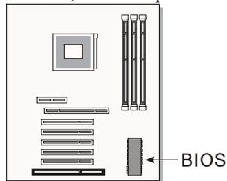
The BIOS IC is inserted in an IC socket, which means that it can be removed and exchanged for another IC if necessary.
