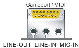
The Gameport can be used with joysticks, or alternatively as MIDI port. The Line-out is for speakers, be sure to use only amplified speakers. The Line-IN and Mic-IN are inputs that can be used for recording.
