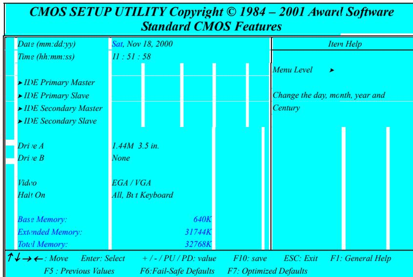
This screen allows you to change the basic CMOS Settings such as date and time, harddisk type etc. After you have made the changes you need to make press [ESC] to return to the main menu.
