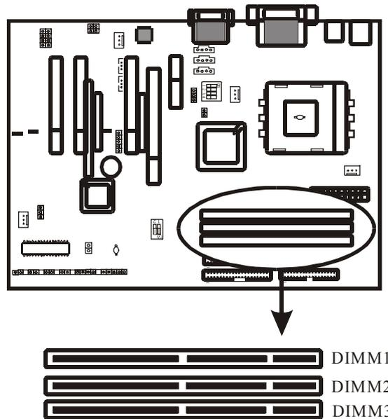
Memory speed is controlled through the BIOS, on the Advanced Chipset Features Setup page you will find several items related to SDRAM speed. Refer to the BIOS section for more details.
