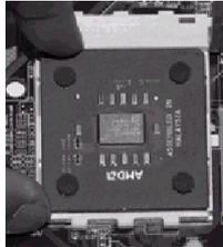
Now with the processor properly installed, you can proceed to install the heatsink. It is important to note that if you have never installed a heatsink on an AMD Athlon or AMD Duron processor before it may be difficult. We recommend you do a dry run a few times before doing the final installation. To allow you to do this read the following instructions. Do not remove the film on the thermally conductive compound until you are ready to do the final installation.
