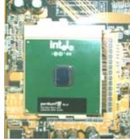
Now with the processor properly installed, you can proceed to install the heatsink. It is important to note that if you have never installed a heatsink on an Intel PIII or Celeron processor before it may be difficult. We recommend you do a dry run a few times before doing the final installation. To allow you to do this read the following instructions. Do not remove the film on the thermally conductive compound until you are ready to do the final installation.
