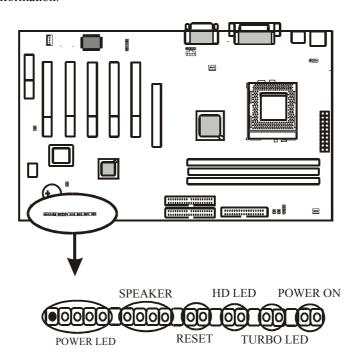
**POWER LED** is a 3-pin connector. It is used to connect to the LED on the case front panel. The LED shows the status of the power.
