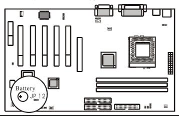
Normally JP12 will be in the 1-2 position, this will connect the battery to the southbridge of the chipset which contains the CMOS memory. If JP12 is temporarily set to 2-3 this will interrupt the battery electricity flow, and the CMOS memory will be erased, this will however only work if the power supply is not switched on. Now at the next reboot the BIOS will automatically load the CMOS default values.
