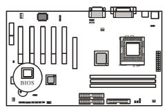
The BIOS IC is inserted in an IC socket, which means that it can be removed and exchanged for another IC if necessary.
