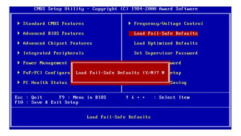
"Load Fail-Safe Defaults" loads optimized settings which are stored in the BIOS ROM. The auto-configured settings only affect "BIOS Features Setup" and "Chipset Features Setup" screens. There is no effect on the standard CMOS setup. To use this feature, highlight it on the main screen and press the <Enter> key. A line will appear on screen asking if you want to load the setup default values. Press the <Y> key and then press the <Enter> key. The setup defaults will then load. If not, enter <N>.
