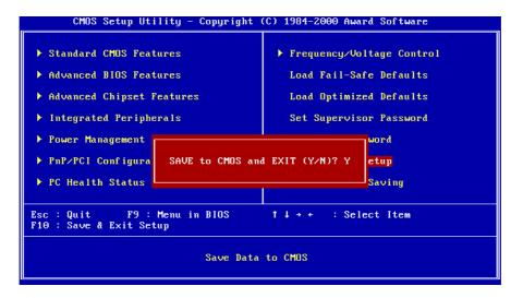
The "Save & Exit Setup" option will bring you back to boot up procedure with all the changes you have made which are recorded in the CMOS RAM.
