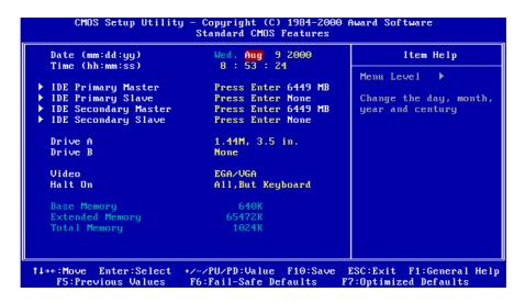
The "Standard CMOS Features" allows user to configure system setting such as current date and time, type of hard disk drive installed in the system, floppy drive type, and the type of display monitor. Memory size is auto detected by the BIOS and displayed for your reference. When a field is highlighted (direction keys to move cursor and <Enter> key to select). The entries in the field will be changed by pressing <PageDown> or <PageUp> key or user can enter new data directly from the keyboard.
