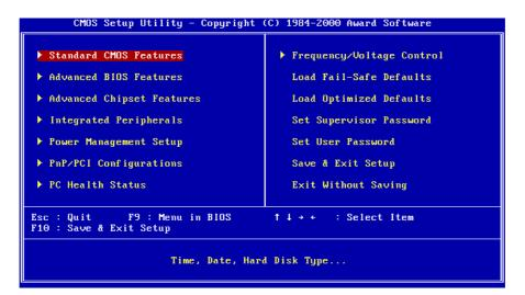
The menu displays all the major selection items and allows user to select any of the shown item. The selection is made by moving cursor (press any direction key) to the item and press **<Enter>** key. An on-line help message is displayed at the bottom of the screen as cursor is moved to various items which provide user better understanding of each function. When a selection is made, the menu of the selected item will appear. So the user can modify associated configuration parameters.
