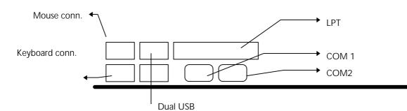
**LPT:** this connector is used to connect parallel port cable.
