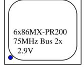
The bottom line of the mark on the processor contains a code 2.9 that identifies the voltage level type. The second line will show the bus MHz and clock multiplier for jumper setting.
