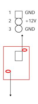
FAN1: CPU cooling fan connector. Wire with +12V voltage (most likely red wire) must be plugged into pin2, and GROUND wires (must likely black wires) must be plugged into pin1and/or pin3. Please confirm the wire color re-presentation with your supplier.
