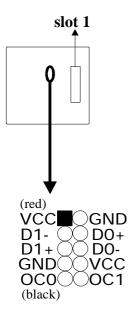
USB : USB connector; Universal Serial Bus; this is used to connect USB devices through an optional dual head cable with an iron plane.
