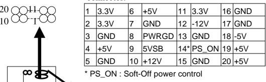
**PW1**: AT mode +5V voltage power supply connector.
