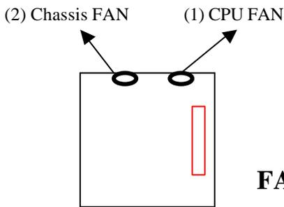
**FAN : CPU cooling fan connector.** Wire with +12V voltage (most likely red wire) must be plugged into pin2, and GROUND wires (most likely black wire) must be plugged into pin3. Please confirm the wire color re-presentation with your supplier.
