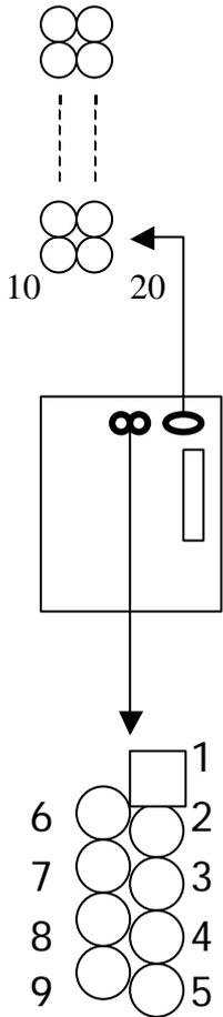
**PW1** : ATX mode +3.3/5/12V power supply connector.
