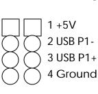
USB connector; Universal Serial Bus; this is used to connect USB devices. There are three connectors on board, user can choice
