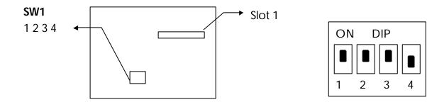
DIP switch, ( ex. : ON,ON,ON,OFF) O N : switch to the 'ON'
