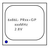
The mark on the processor is shown as a sample on the left. The code-name 6x86L is dual voltage mode processor.
